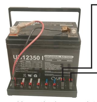
12 volt battery with Anderson PowerPole Connectors can power both LHG 5 and WiFi Router.
