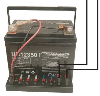
12 volt battery with Anderson PowerPole Connectors can power both LHG 5 and WiFi Router.
